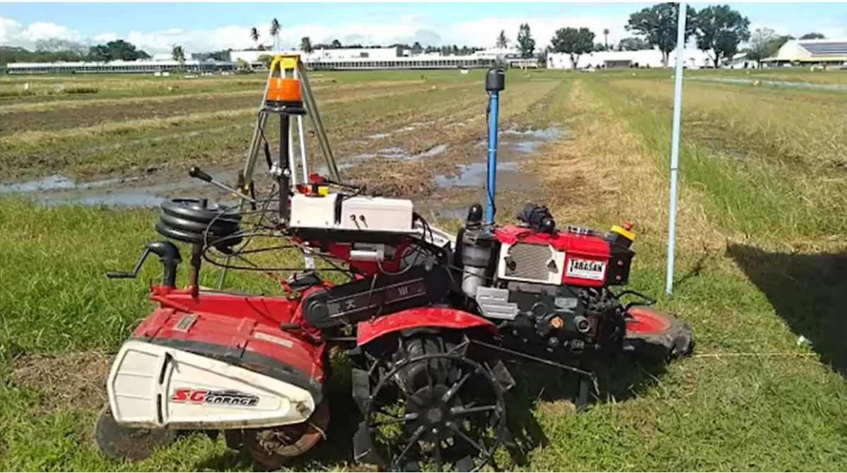
Agrotis RoboTractor unit with metal cage wheels for better movement across rice paddies
