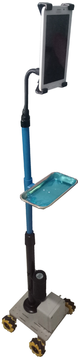
The Logistic Indoor Service Assistant (LISA) with independently driven Mecanum wheels and adjustable holder
